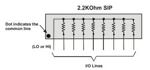
Figure 4. Eight-resistor SIP schematic
